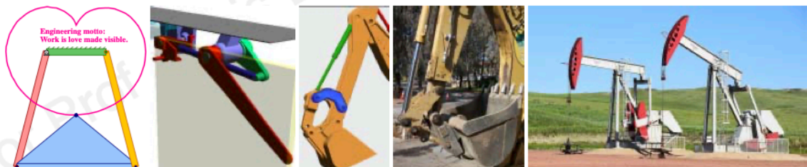
Examples of 4-bar linkages: Courtesy Design Simulation Technology (SimWise)
